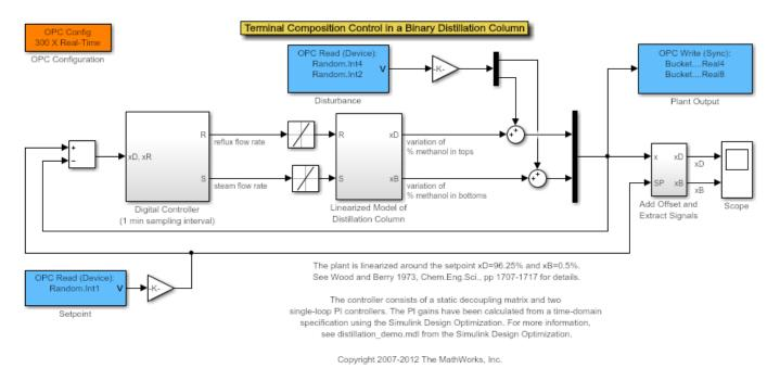
The distillation column controller has been tuned using Simulink® Design Optimization<sup>™</sup>. For more information, see distillation\_demo.mdl from Simulink Design Optimization.
